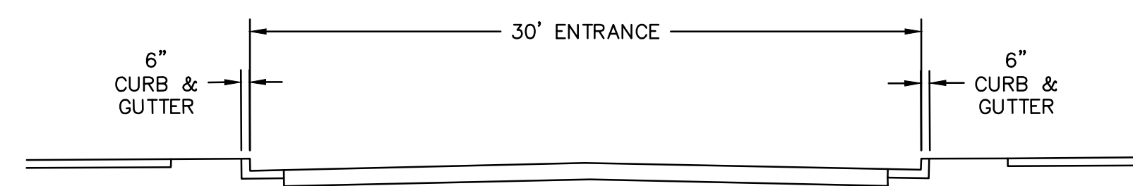
TYPICAL ENTRANCE SECTION B-B NTS
